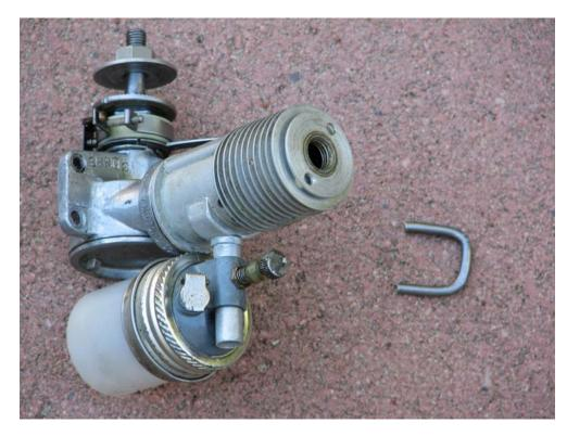
The U shaped spanner tool is placed in a vise with just a short section of the two legs protruding.
